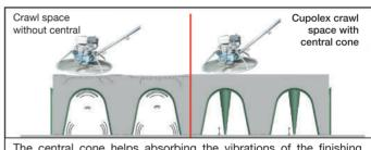
The central cone helps absorbing the vibrations of the finishing procedure, preventing the formation of microcracks
